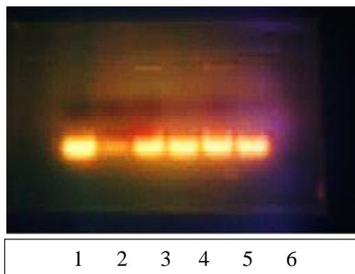
Lane 1(C) –Herring sperm DNA damaged with hydroxyl radical from Fentons reagent.
